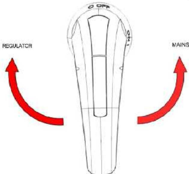
3. Turn the inlet switch to ON position.
