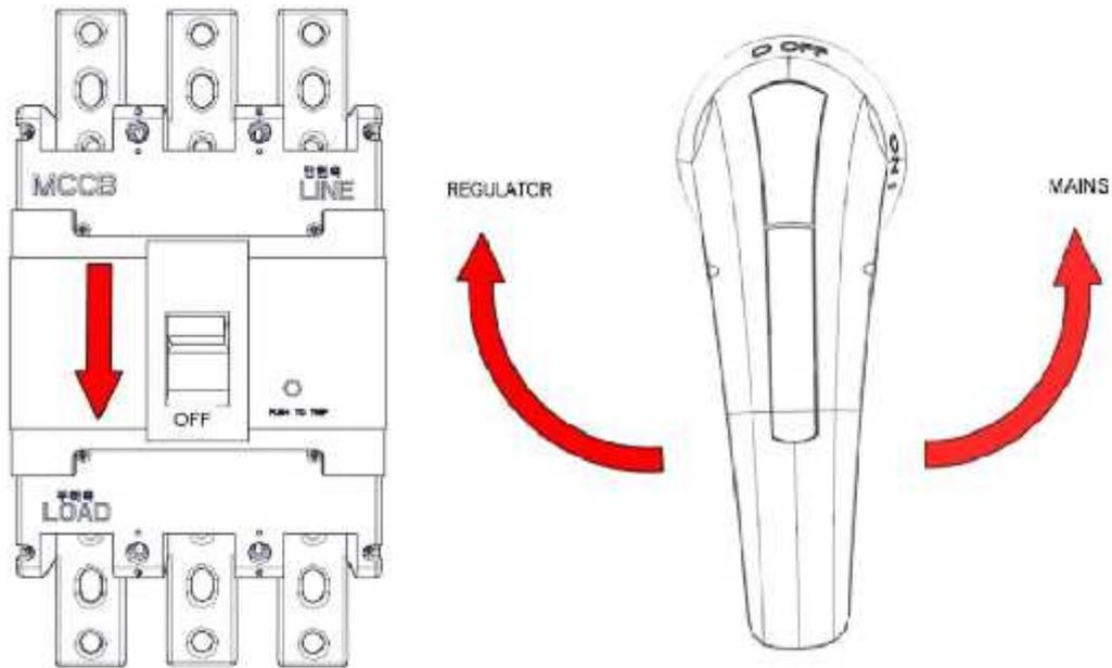
The inlet and bypass switch are at OFF position.
