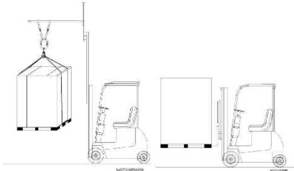
All MRG/MSR33 series servo voltage regulator cabins are delivered on transportation pallets.
