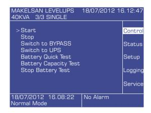
Some menus have changeable options like ON/OFF, duration or quantity. To make changes in the menu press ENTER to choose the variable, up and down keys to change the value, and press ENTER to set the new value. Press ESC to cancel.
