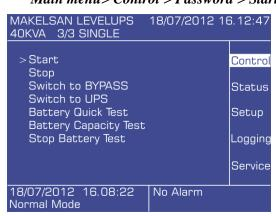
5. Check the UPS has switched to normal operation mode, via mimic diagram LEDs and LCD panel.
