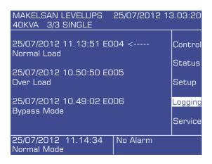
When viewing a log, press enter to see detailed info about the UPS. All recorded data for that particular event (status, setup etc.) can be seen on the menu.
