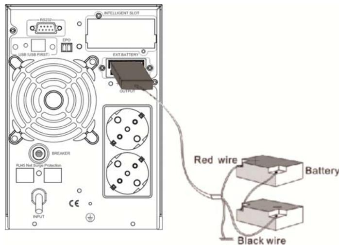
**FIG.7 battery connection**
