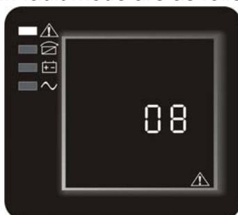
Fault mode (LCD interface on which the fault code display)
