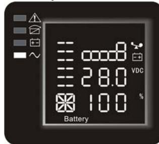
Battery remaining time: Display the battery remaining time when under battery mode. The number is from 0 to 999 minutes. As the following graphics shown: there are 686 minutes left for discharging.
