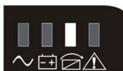
Bypass yellow LED is on, the buzzer beeps once every 2 minutes . The warning red LED is on when beeping, LCD displays are according to the exact load and battery capacity.
