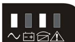
When the input mains meets the input range of the ECO mode and start the ECO function, the UPS will works on ECO mode. If input AC mains exceeds the range of ECO several times in a row in a minute but stays in inverter input range, UPS will work on AC inverting mode automatically.
