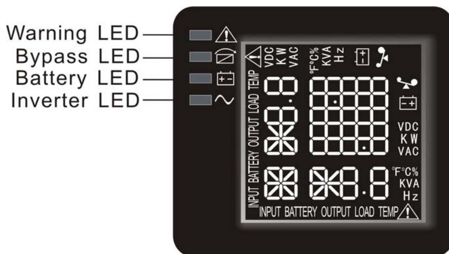
Warning red LED is on: UPS is fault. For example: Overload beyond the allowed time, inverter fault, BUS fault, over temperature fault etc.
