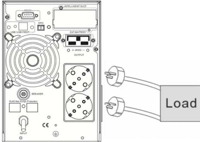
**FIG.6 Output connection**
